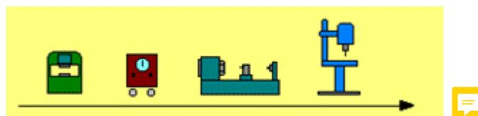
Here equipment is laid out according to the **processing sequence**, irrespective of the typology of machinery involved. What is important is:
