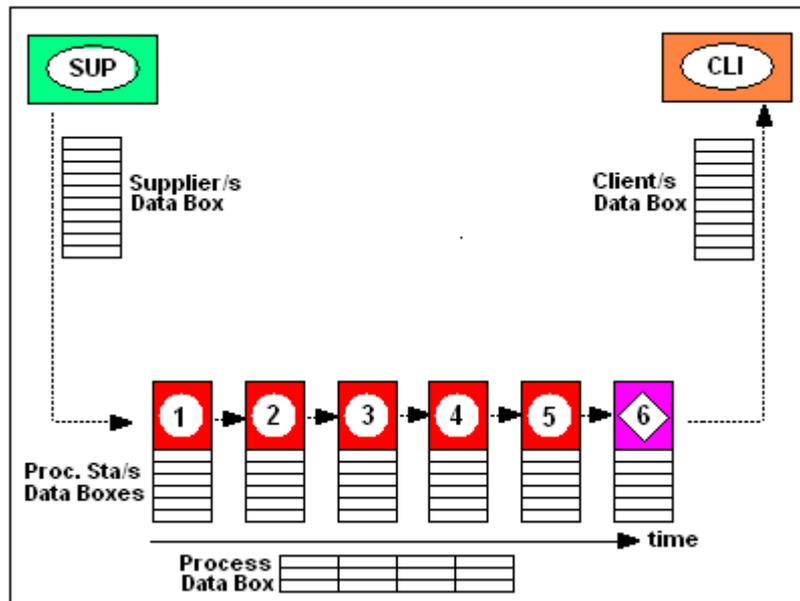
Note: attached to each Processing Station icon there is a **data box** (which must then be filled with data). A similar one is drawn next to Supplier and Client icons. Also a data box regarding the entire process is positioned in the Current State area.
