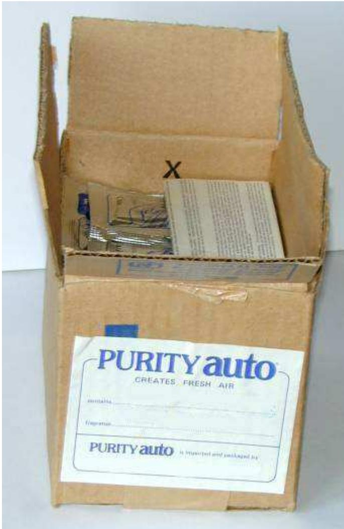
b.1) Packaging 50 Sachets into a Carton of 50 consists of: preparing Cardboard Box - counting 50 sachets (one fragrance or assorted) and inserting them into the Cardboard Box with instruction leaflet and Packaging Labourer tag - closing cardboard box with sealing tape - and storing it (buffer stock) on shelves. The associated cycle time is approx. 45" for one fragrance carton and 60" for assorted fragrances.
